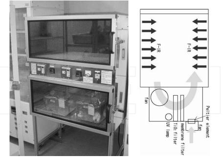
Figure 8. The FIR animal raising apparatus
