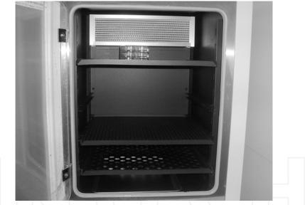
Figure 7. The FIR CO2 incubator
